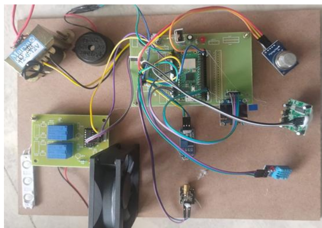
Fig. 4.2. Working Model of IOT-Based Household equipment control system using LASER-LDR pair
